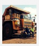
5800 operation hours 95% mechanical availability 500 000 total tonnage 49 l\hour fuel consumption
